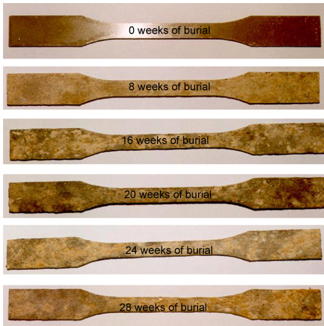
Fig. 7. Pictures of different stages of biodegradation of flax/PHB/HV (8 wt.%) composites with 20 vol.% fibre after burial in soil.
